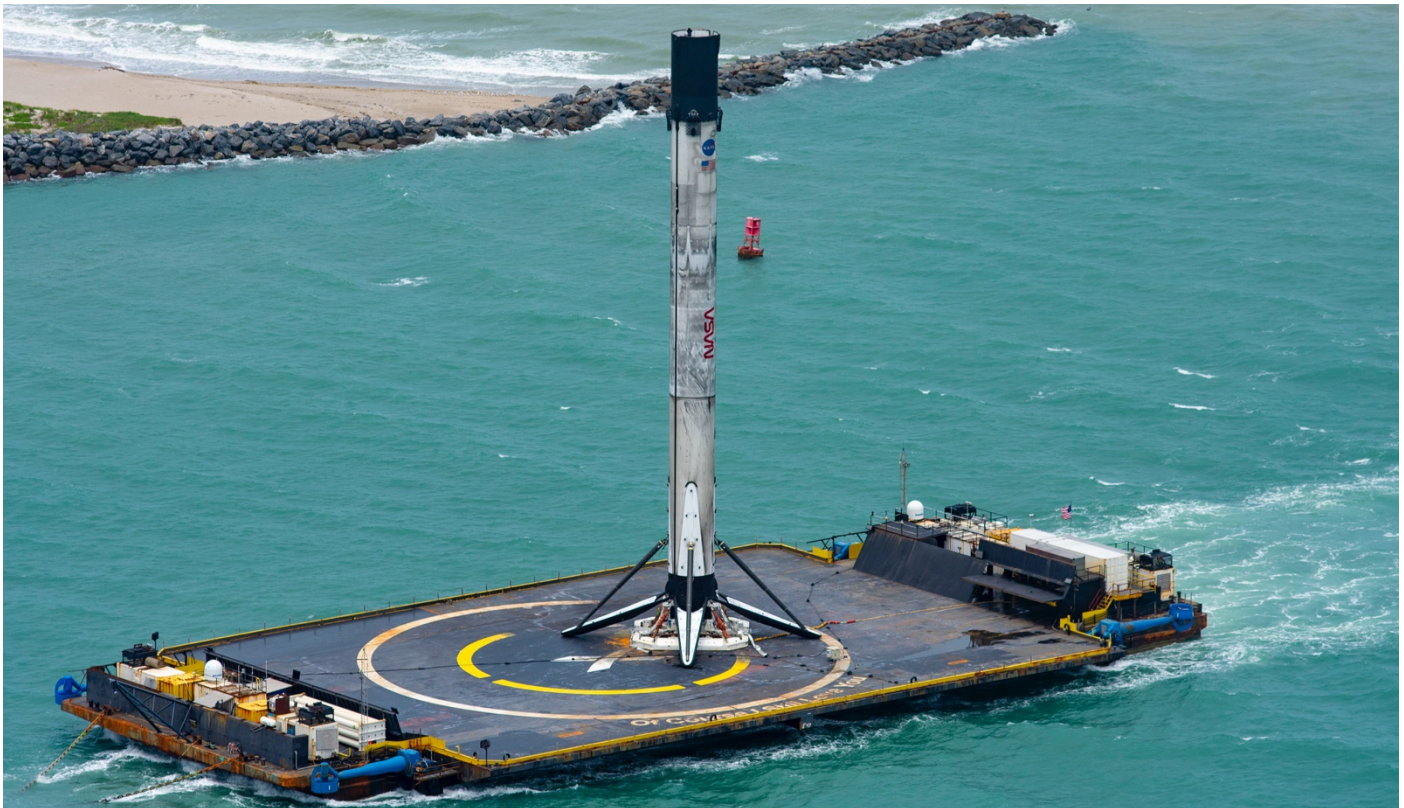
Figure 21 SpaceX Falcon 9 first-stage booster successfully landed on the autonomous spaceport drone ship (ASDS) "Of Course I Still Love You" in the Atlantic Ocean, following orbital launch. The booster utilizes landing legs and grid fins for controlled descent an.
