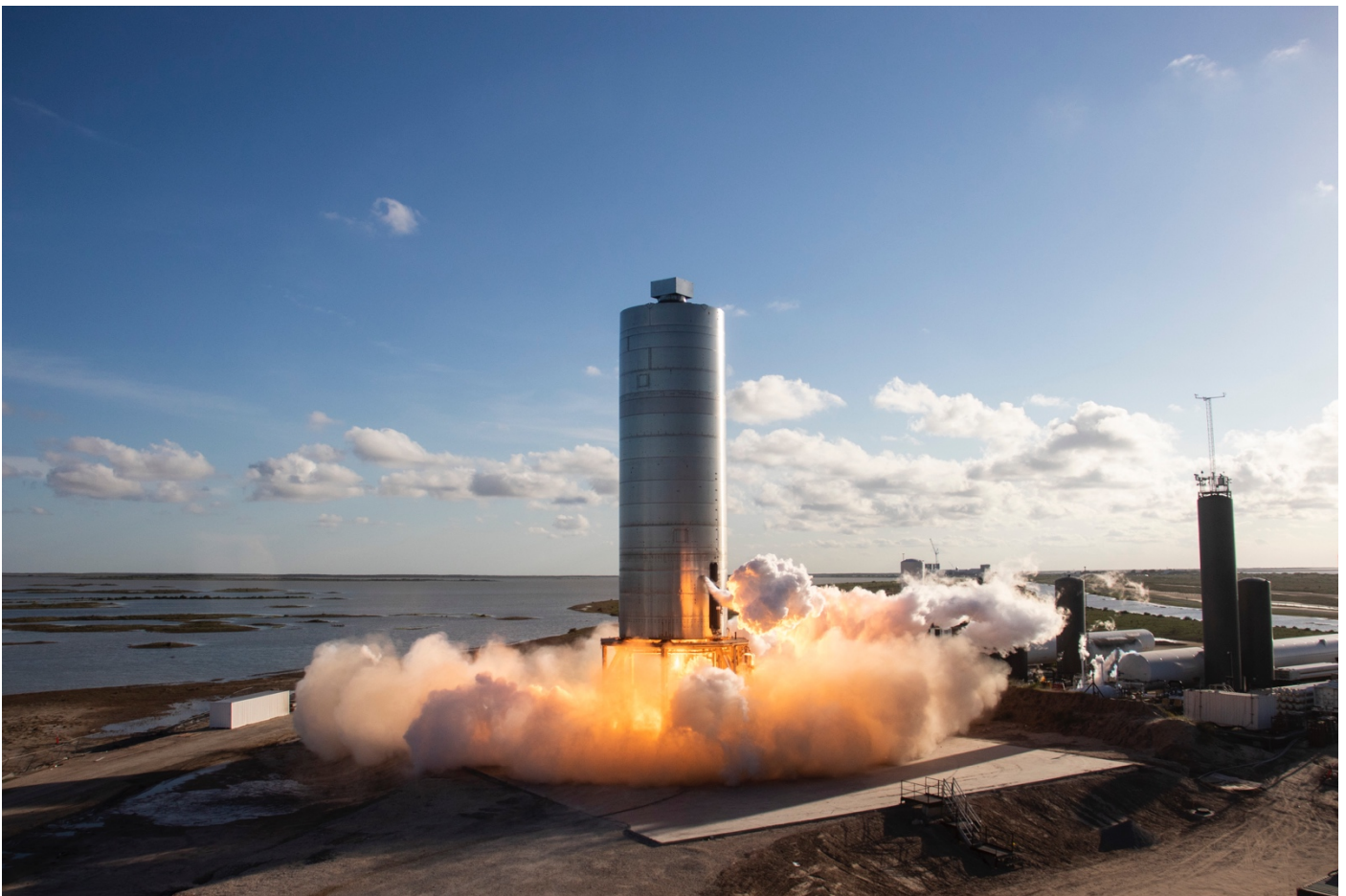
Figure 22 SpaceX Starship SN5 prototype conducting a 150-meter hop test at the SpaceX Boca Chica launch facility, utilizing a single Raptor engine powered by liquid methane ( \text{CH}_4 ) and liquid oxygen ( \text{LOX} )
