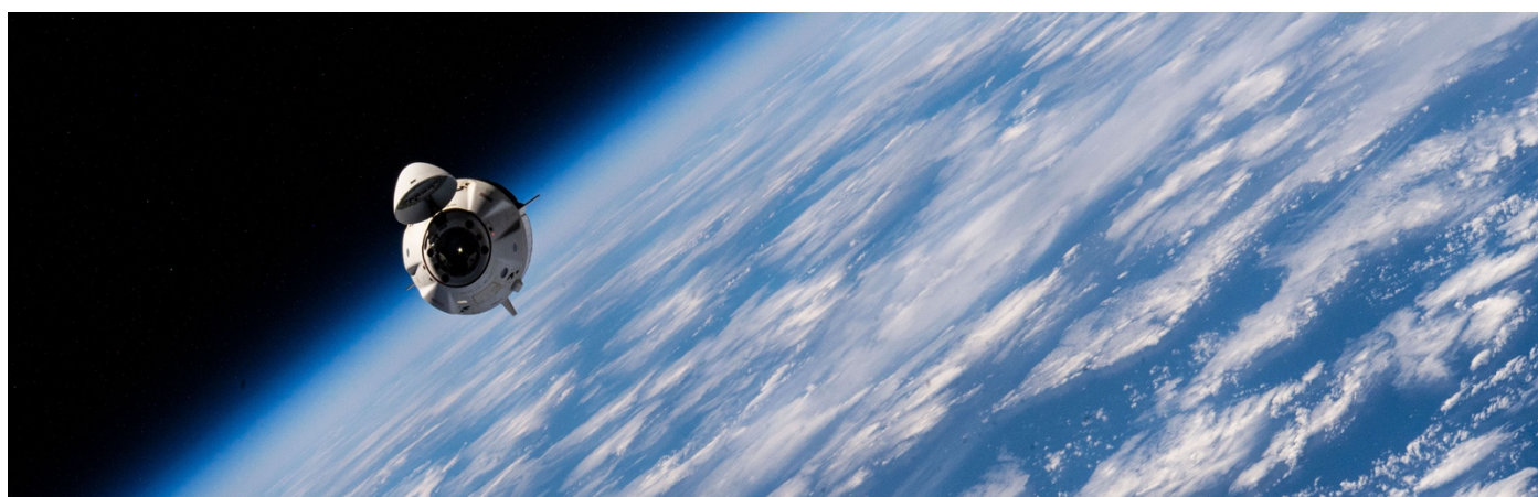
Figure 7 SpaceX Crew-2 Return Mission Dragon spacecraft in low Earth orbit approaching the International Space Station, with its nose cone open in preparation for docking operations
