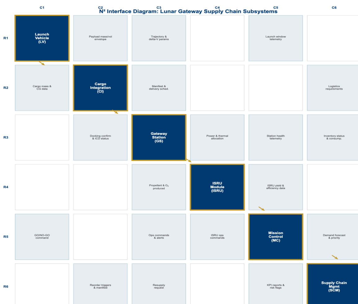
Figure 10 N 2 Diagram - Supply Chain Function Interface Matrix (F-1 through F-6). Bold entries indicate primary inter-function data or material flows; shaded diagonal represents self-contained function processing. Find this image detailed interaction in appendix
